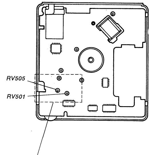
On this set, it is very difficult to simplify this adjustment. For those sets on which symptoms such as "occasional skipping" are hard to discover, or it is hard to tell if the set has been repaired, use the CD jig and perform this adjustment. Refer to the diagram below for connection of the CD jig. The adjustment procedure is described in the separate CD Jig Instruction Manual.
