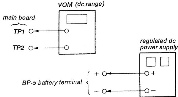
1. Connect VOM to TP1 and 2 on the main board and supply 3.92 Vdc to BP-5 battery terminal. (At this time, supply 9 Vdc to the external power supply jack (DC IN 9 V).)
