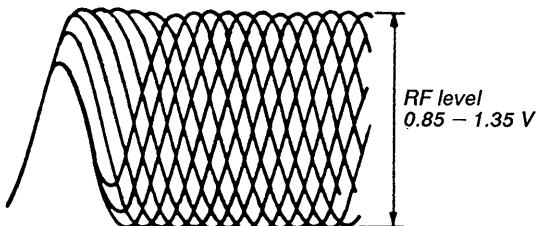
When observing the eye pattern, set the oscilloscope for AC range and raise vertical sensitivity.
