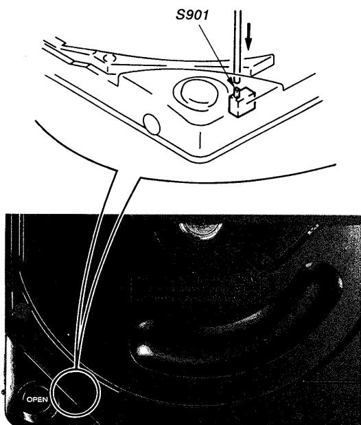
*Fig. 1 Turning S901 Connection*
