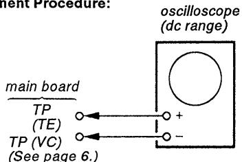
1. Connect the oscilloscope to servo board TP (TE).
