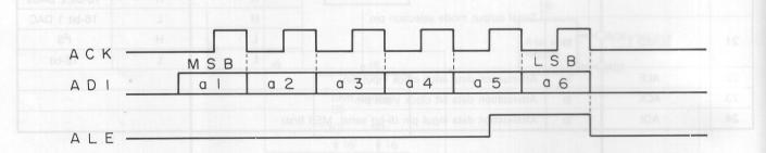
The setting of the attenuation data on the above timing can be performed asynchronously with the digital filtering. In addition, when the  $\overline{\rm ATT}$  pin is made ''H'' (or open), the attenuation data is reset and the digital attenuation goes OFF.
